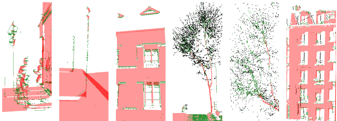
Figure 14. Comparison of the three methods: the naive filtering, the edge filtering and its extension with the triangle filtering. From left to right, the scenes represent: a person pushing a stroller on a pavement, two poles, the top of a facade, a tree, a zoom on the tree's foliage, a facade in the grazing surface case.
